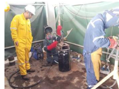
Welder Qualification Test (WQT)
